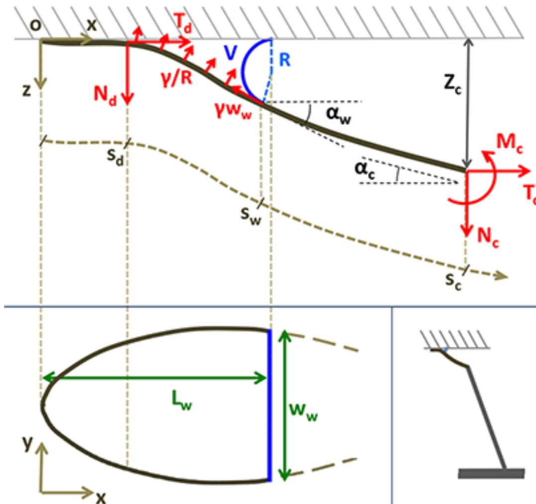
Diagram of the forces applied to the hair tips (dark grey line) located on the feet of the insect.
